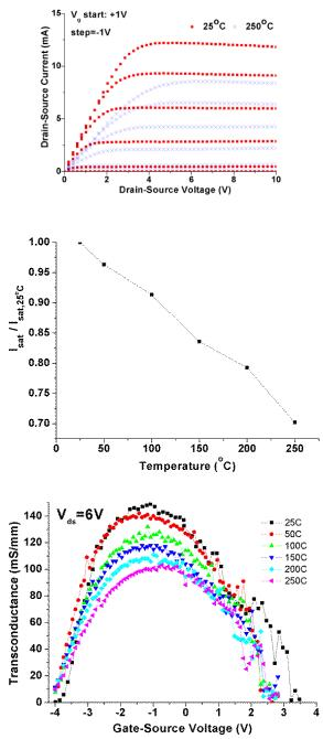
Figure 2. Measured saturation current at  $V_g=0V$  as a function of the ambient temperature. The data are normalized to the current value at room temperature.
